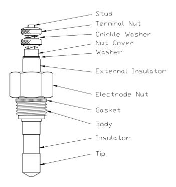
Figure 4.1 - Low pressure electrode
